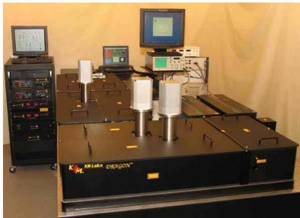
Figure 3. KMLabs RedDragon laser system that produces 25 W, 25 fs at 5 kHz. This system includes Carrier Envelope Phase stabilization.
